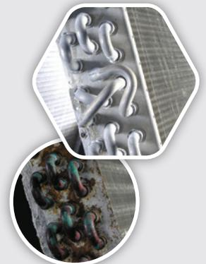
Traditional copper and galvanized steel coils are highly susceptible to corrosion.
